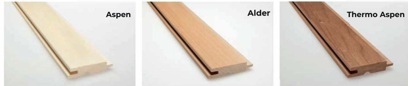
15x70 | Thickness: 15 mm | Width: 70 mm | Effective width: 57 mm | Use per square meter: 17,5 m | Package: 6 pcs
