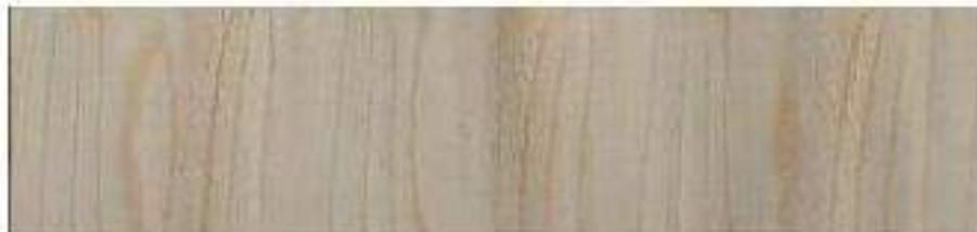
A low density veneer good for structural plywood core only
