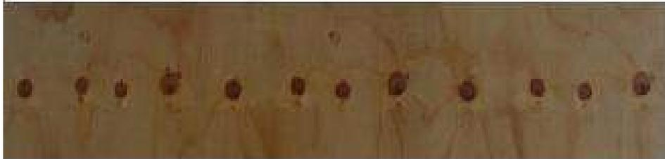
Nearly critical section with almost 1/4 of the veneer width covered by defects
