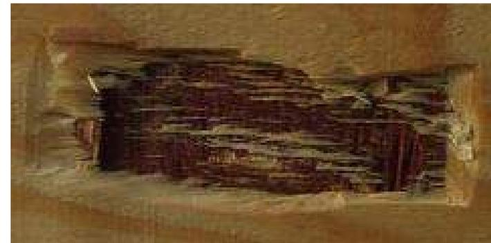
An unacceptable knife test example,
