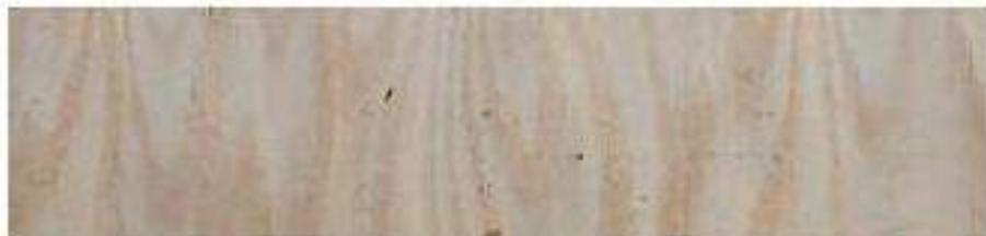
A medium density Veneer good for Structural plywood faces and backs
