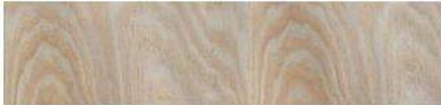
A high density veneer good for LVL and also excellent for structural plywood faces and backs
