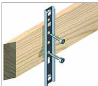
Attach the facade clip using the profile screws.
