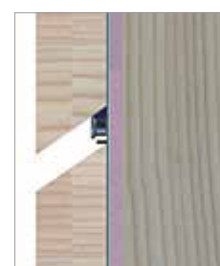
The size of the dilatation gap will be automatically set by the head of the screw. Done!
