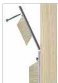
Simply slide the next profile in and attach only at the top using a screw.
